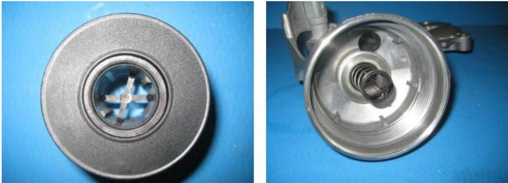
The two photos above show the filter MD-525 and the housing. If you notice the filter, you will see that in its center there is a cross. In the center of the housing you will notice a spring loaded valve. That valve separates the two different paths that the oil can flow to. When the valve is up (No filter installed) the oil flows back to the sump, so during the oil change the housing empties of oil.
