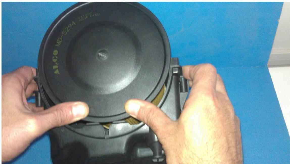
3. After the filter passes behind the 2 clips it is secured in place.
