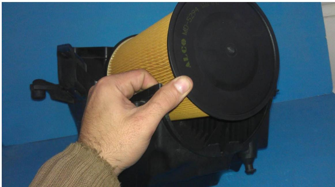
2. To secure the filter in the housing, you need to lift the filter a little, so that it is above the clips and then push it like it is shown in the photo below so that it passes behind the clips.
