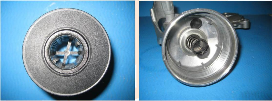
The two photos above show the filter MD-525 and the housing. If you notice the filter, you will see that in its center there is a cross. In the center of the housing you will notice a spring loaded valve. That valve separates the two different paths that the oil can flow to. When the valve is up (No filter installed) the oil flows back to the sump, so during the oil change the housing empties of oil. When the valve is down (Filter installed) the oil flows to the engine to lubricate it.
